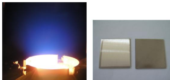
Figure 1: The plasma source and thin films deposited on stainless steel
