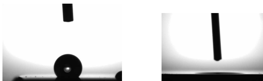
Figure 1: Water droplets on plasma polymerized surfaces. (a) shows a surface containing a high amount of nanoparticles. (b) shows the same surface after post process plasma treatment.
