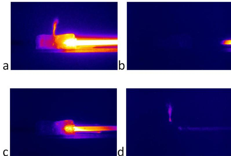
**Figure 1:** Plasma bullet propagation in agarose gel with an L-type tube: images taken with a high-speed ICCD camera a) exposure time 20  $\mu\text{s}$  b-d) exposure time 100 ns, delays b) 0.3  $\mu\text{s}$ , c) 0.6  $\mu\text{s}$ , and d) 1.5  $\mu\text{s}$ .
