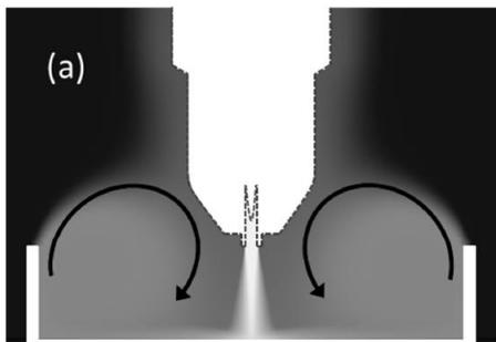
Fig 1: Flow Simulation of ambient species densities in plasma jet treatment in a petri dish [4]
