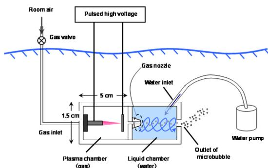
Figure 1 Experimental setup of P-MS.
