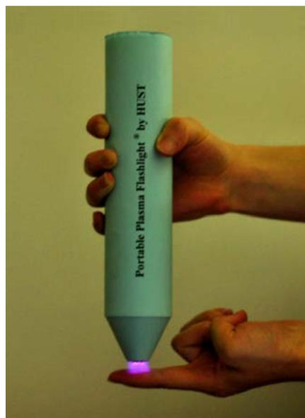
Fig. 1. Photograph of the air plasma flashlight
