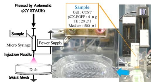
**Figure 1:** Experimental setup.
