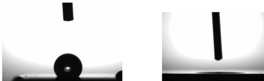
**Figure 1:** Water droplets on plasma polymerized surfaces. (a) shows a surface containing a high amount of nanoparticles. (b) shows the same surface after post process plasma treatment.
