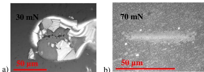
**Figure 1:** Results of wear tests a) destroyed SiO<sub>x</sub>-layer on polished enamel, b) wear resistant SiO<sub>x</sub> layer skid mark on phosphorus acid pre-etched enamel
