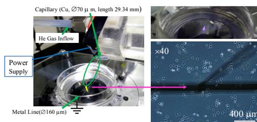
**Figure 1:** Experimental setup.
