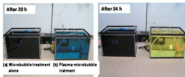
Figure 2 Indigo Carmine solution after the P-MB treatment.
