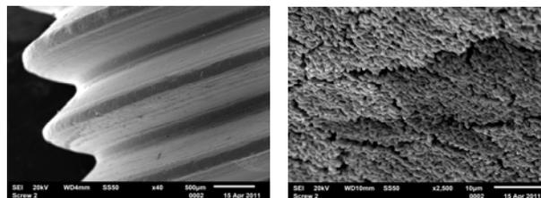
**Figure 1:** SEM images of the contaminated screws
