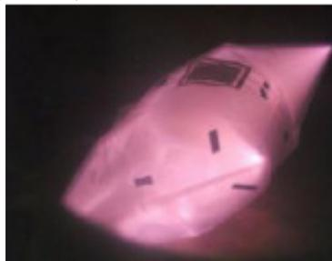
**Figure 1:** Generated plasma inside the packaging bag
